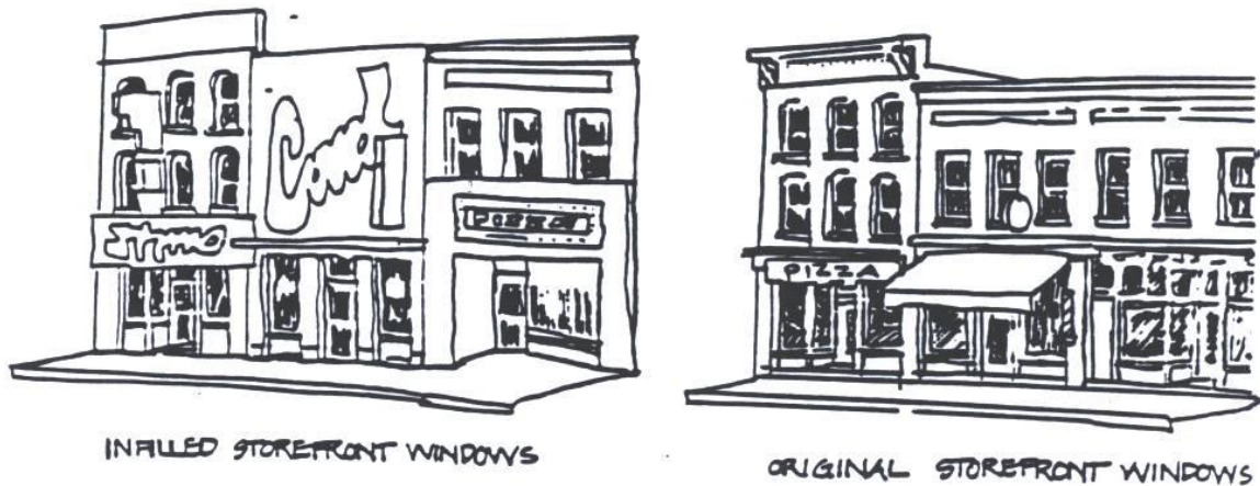
Illustration 20.2 Avoid Attempts at Hiding an Older Façade.
